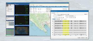
The unique AMI Marine Replay software provides 'Audio Scan' and 'Jump to Incident' functions to provide intuitive data review by engineers, ship's crew, accident investigators and even for crew training purposes.
